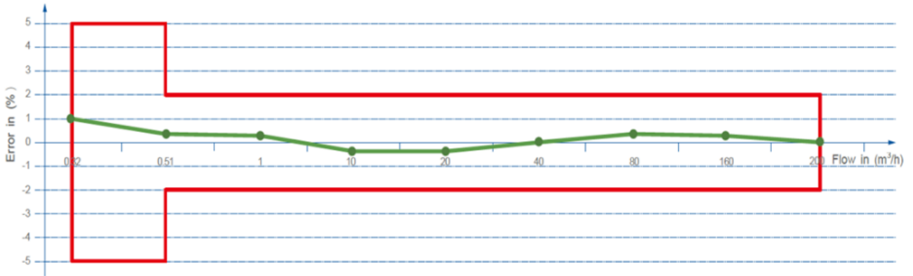
Meter performance curve DN100
